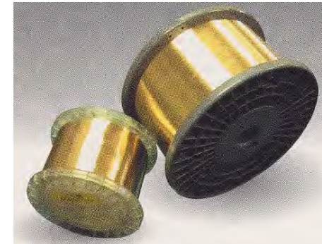
Machinable Cu-40%Zn-3.2%Pb alloy
