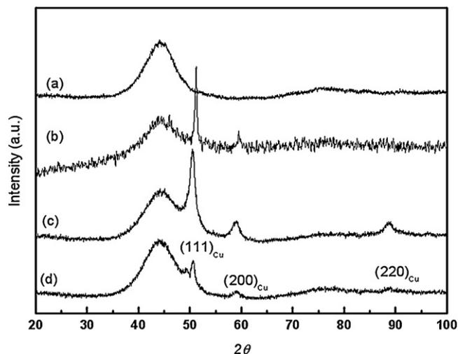
Fig. 2. XRD curves of the HPT processed sample and the as-cast  $Zr_{55}Cu_{30}Ni_5Al_{10}$  BMG. (a) As-cast BMG, (b) 10, (c) 20 and (d) 50 HPT rotations.
