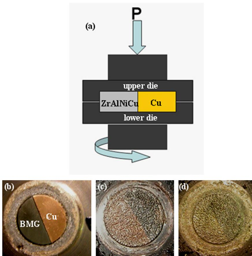
Fig. 1. (a) Schematic illustration of the HPT process and the appearance of the BMG/Cu sample (b) before and after HPT process with (c) 20 and (d) 50 rotations.
