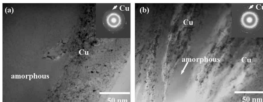
Fig. 4. TEM images showing the microstructure of the HPT processed sample with different rotations. (a) 20 rotations inserted with SAED pattern and (b) 50 rotations inserted with SAED pattern.
