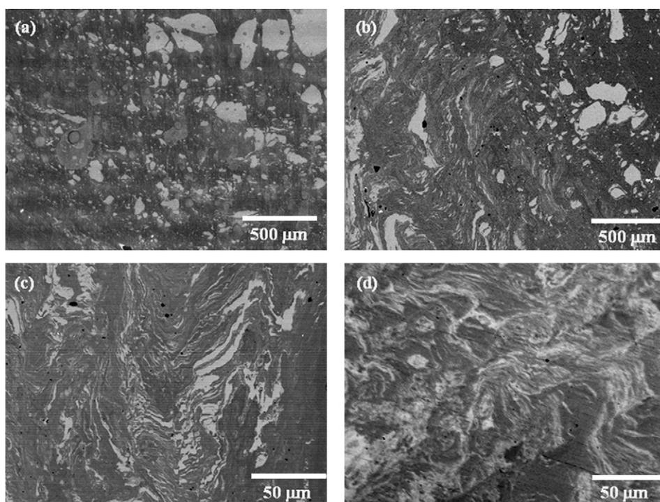
Fig. 3. SEM-BSE images showing the microstructure of HPT processed samples with (a) 10, (b) 20 and (d) 50 rotations.
