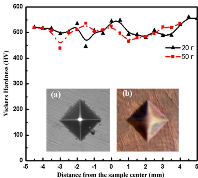
Fig. 5. Vickers hardness profile across the sample HPT processed with 20 and 50 rotations, inserted with the appearances of the indent of (a) monolithic BMG and (b) HPT processed BMG/Cu with 50 rotations.
