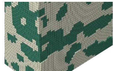
Fig. 6 Slip deformation at Fe/Mg interface.
