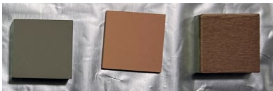
Figure 1. Photo of specimens used in this study. Specimens from left to right are: SUS304, p-Cu, LC-Cu.
