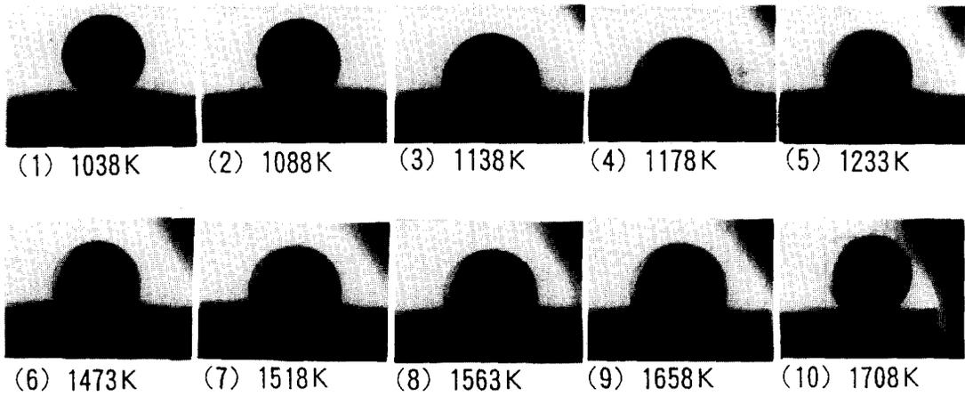
Fig. 7. Change in shape of liquid tin on diamond (110) with temperature in argon-10% hydrogen atmospheric gas.
