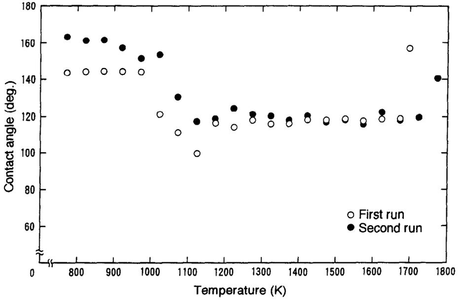
Fig. 5. Variation of contact angle between liquid tin and diamond (111) with temperature in argon-10% hydrogen atmospheric gas.
