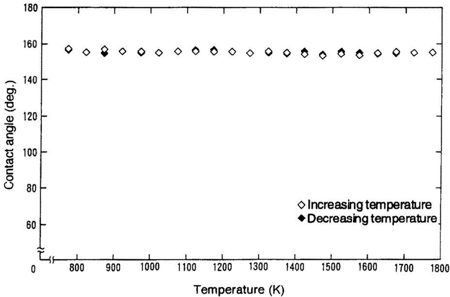
Fig. 9. Effect of temperature hysteresis on contact angle between liquid tin and graphite.
