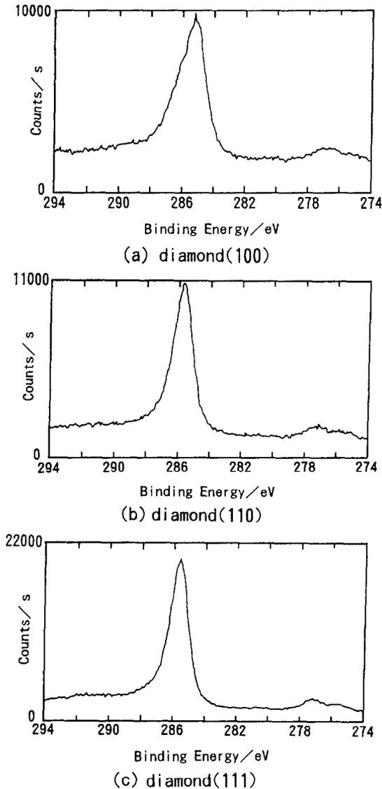
Fig. 4. XPS spectra of diamond surface heated at 1723 K.
