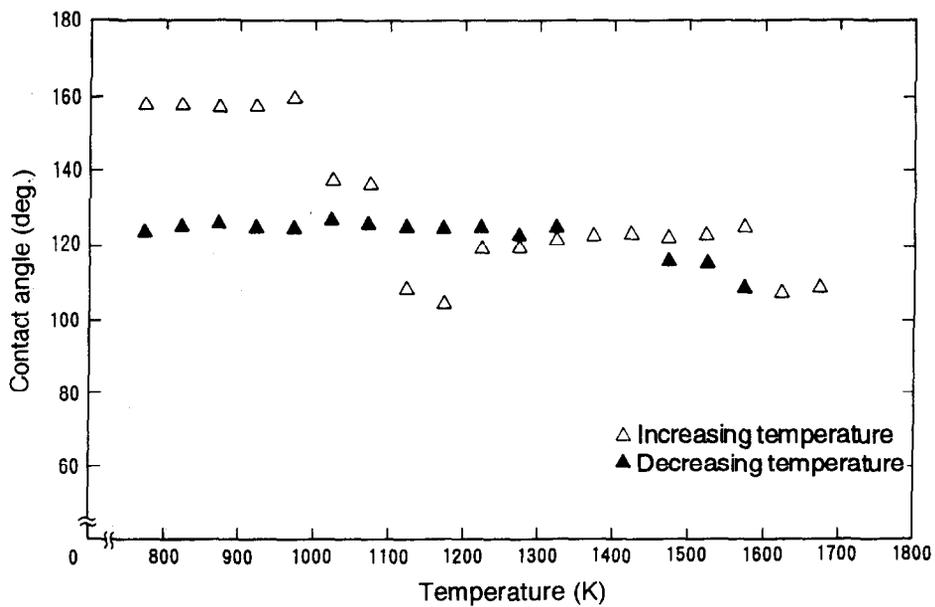
Fig. 8. Effect of temperature hysteresis on contact angle between liquid tin and diamond (110).
