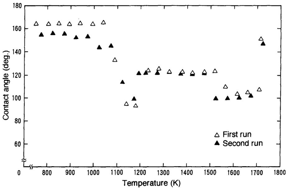
Fig. 6. Variation of contact angle between liquid tin and diamond (110) with temperature in argon-10% hydrogen atmospheric gas.
