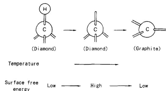
Fig. 3. Change in surface condition of diamond with temperature.
