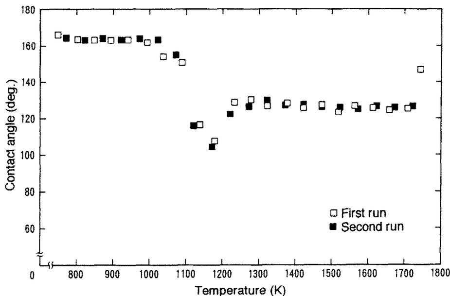
Fig. 2. Variation of contact angle between liquid tin and diamond (100) with temperature in argon-10% hydrogen atmospheric gas.
