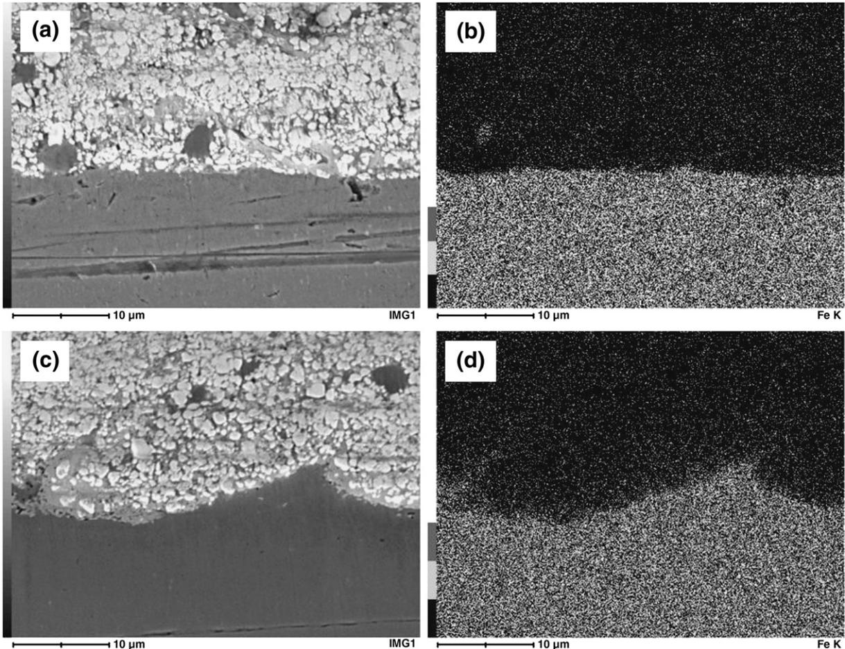
**Fig. 9.** SEM images and Fe mapping images of the boundary between the WC–Cr–Ni layer and the substrate. (a) SEM image of the as-sprayed sample, (b) SEM image of the FSPed sample, (c) Fe mapping image of the as-sprayed sample, and (d) Fe mapping image of the FSPed sample.
