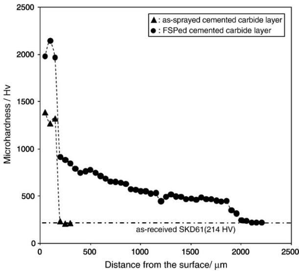
**Fig. 8.** Microhardness depth profiles of the cross-section of the as-sprayed and the FSPed WC–Cr–Ni layer.
